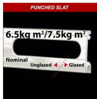
The Ra4 Punched Curtain provides 44% vision. It uses a 40mm high single skin aluminium lath, with 100mm x 20mm slots. The punched laths can be mixed with Solid Laths to provide a more secure option. For added security there is also the option for polycarbonate inserts. The punched lath is only available up to 3m wide shutters, over 3m wide only 4 laths can be punched.
