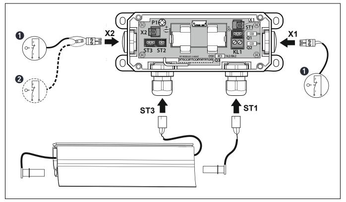
● Slack-rope switch ● Pass-door switch
