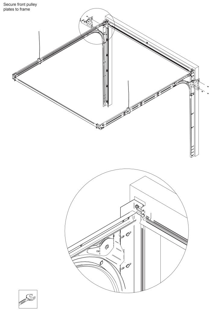
Measure from corner to corner to determine if the horizontal track area is square, adjust accordingly. Before securing the L shape hangers, ensure the horizontal tracks are level
