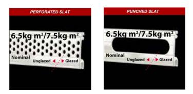
The Ra4 Punched Curtain provides 44% vision. It uses a 40mm high single skin aluminium lath, with 100mm x 20mm slots. The punched laths can be mixed with Solid Laths to provide a more secure option. For added security there is also the option for polycarbonate inserts. The punched lath is only available up to 3m wide shutters, over 3m wide only 4 laths can be punched.
