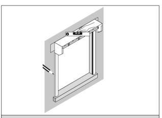
**4** Offer the shutter to the opening and centralise, ensuring the top of the shutter box is horizontal and that both guide rails are vertical. Mark the guide location.
