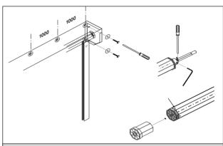
10 Fit the shutter box using the recommended fixings and spacings. Once the shutter box has been installed check the dummy end making sure that it is securely located within the axle. If the dummy end is a shaft bolt design make sure that the centre shaft is fixed in place so that it can not slide back into the axle.
