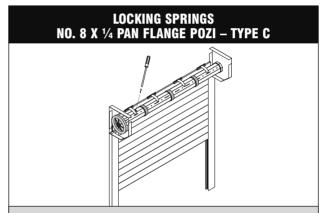
16 Before you attach the curtain to the axle you should determine where you will mount the winder then pull the belt wrapped around the drive wheel so that the belt will pass the winder by at least 400mm. Attach the locking springs to the axle using the screws supplied.
