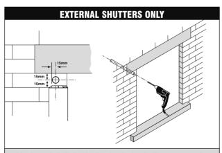
5 Mark and drill the belt tube hole. Drill a 10mm pilot hole followed by a 22mm hole for the tube.
