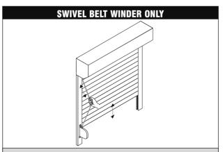
**24** Test the operation of the winder and the shutter to ensure that the belt feeds into and out of the winder correctly and also that the shutter moves freely up and down in the guide rails.
