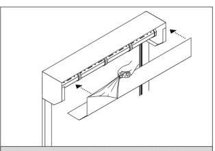
**17** Remove the protective film from the box lid then fit the box lid to the shutter box. If the shutter is externally fitted the box lid should be fastened using appropriately coloured 4mm rivets.
