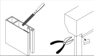
2 File the top of the guides at an angle to create the optimum lead in for the curtain. Guide insert should also be trimmed to suit the filed guide top and securely crimped in place. If the shutter is being face fitted remove the lip from the box back which overlaps the guide rails.
