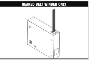
**22** Load the belt into the winder. The belt will be supplied to the correct length. Take off the front of the winder, pass the belt between the rollers and fasten by knotting securely into the centre of the large cog. Reassemble the winder before fastening to the wall.
