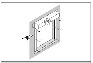
**27** To complete the installation you should fit cover caps to the guide rails (if applicable), mastic around the edges of the shutter then give the shutter a final clean and tidy.
