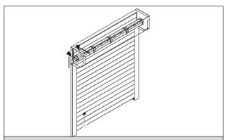
**26** Test the shutter to ensure that the curtain locks correctly when the curtain closes fully. Please refer to the operating and maintenance instructions supplied for the correct method for operating and locking the shutter.
