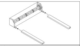
**3** Carefully locate the guide rails fully onto the box lugs ensuring that on face fit guides the 13mm holes are on the outside. When moving the shutter as a complete unit you should minimise the movement of the guide rails to prevent the locating lugs from being snapped of the shutter box. If the shutter is too large to be lifted up as a complete unit you should offer up, locate and fix the individual guide rails then the shutter box.
