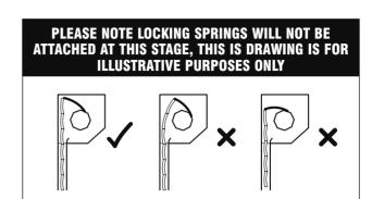
14 Check the curtain height. When pushed towards the back of the shutter box the curtain should finish just under the box top. If the curtain is too tall then slats should be removed to obtain the correct height. If the curtain finishes more than one slat beneath the shutter box top then the curtain is too short and the height must be increased in order for the shutter to lock correctly when fully down.
