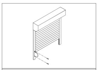
**23** Mount the winder at a convenient height for operation either to the wall or to the guide rails as appropriate.
