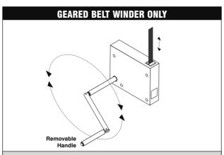
**25** Test the operation of the winder and the shutter to ensure that the belt feeds into and out of the winder correctly and also that the shutter moves freely up and down in the guide rails.
