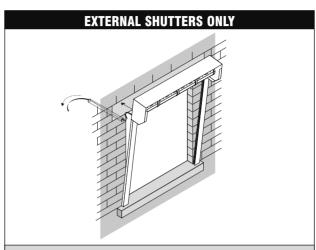
8 Unwind belt and feed through tube whilst offering the shutter to the opening
