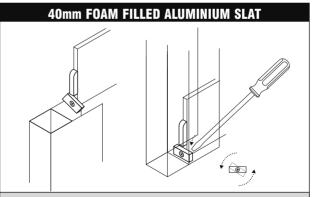
12 If adjustable T stops have been fitted in the bottom slat they should be set to an angle of approximately 45° to enable the bottom slat to enter the top of the guide rail. Once the bottom slat has entered the guide rail the T stop should be set to the horizontal position to prevent the curtain from being accidentally lifted out of the guide rails.
