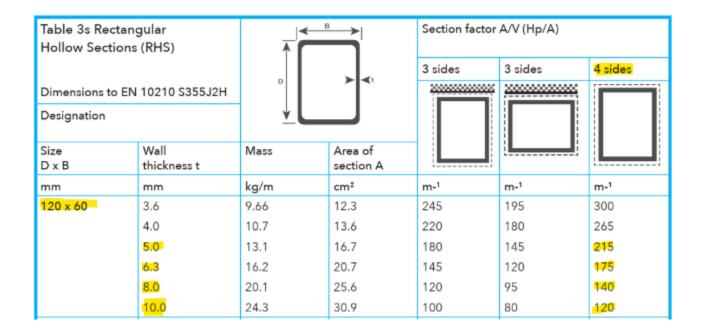
The example above demonstrates that only a 120 mm x 60 mm rectangular hollow section (RHS) with a thickness of 5 mm, 6.3 mm, 8 mm or 10 mm would be suitable as the calculated sectional factor is less than the stated 230m-1 as required within Extended Application Rule J.2.1.
