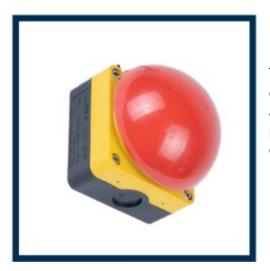
The emergency 'red mushroom' button, which can be operated by palm or foot, can be connected to the FCP03 audio-visual control panel and upon the button being pressed the fire shutter can be programmed to open or close. Typically, utilized as emergency open buttons.
