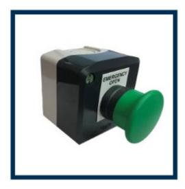
The 'Emergency open' push button can be connected to the FCP03 audio-visual control panel and upon the button being pressed the fire shutter can be programmed to 'open'. Once pressed and the door opens for several minutes, then the FCP03 panel will begin a close cycle once more.
