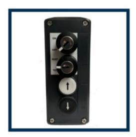
This device allows the trained user to isolate the control functionality locally; it also allows the user to undertake a controlled simulation of fire conditions. This push button station includes a 'reset' function which allows the user to test and then reset the control panel and fire-resistant roller shutter. This is ideal for fire shutters installed in schools, as the access to the fire shutters controls can be locked to stop unwanted operations.
